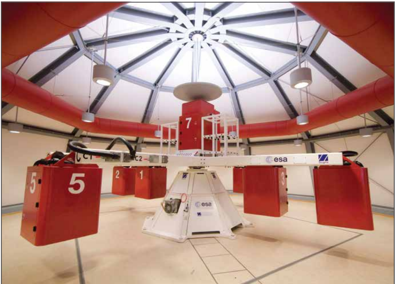
Image 2-1: The Large Diameter Centrifuge at ESA-ESTEC
