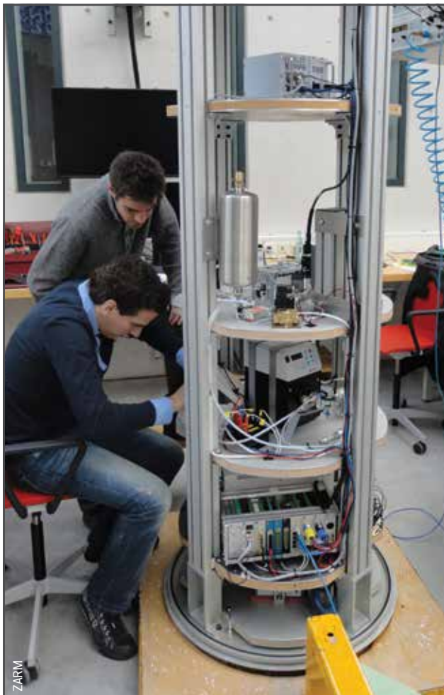
Image 4-2: Integrating an experiment in the drop capsule
