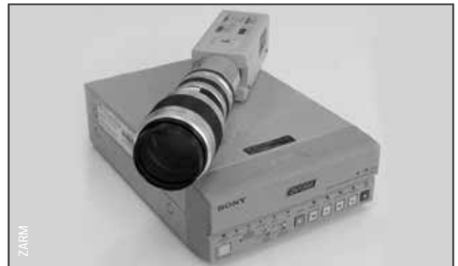
Image 4-4: DVCam™ recorder and CCIR camera with zoom lens
