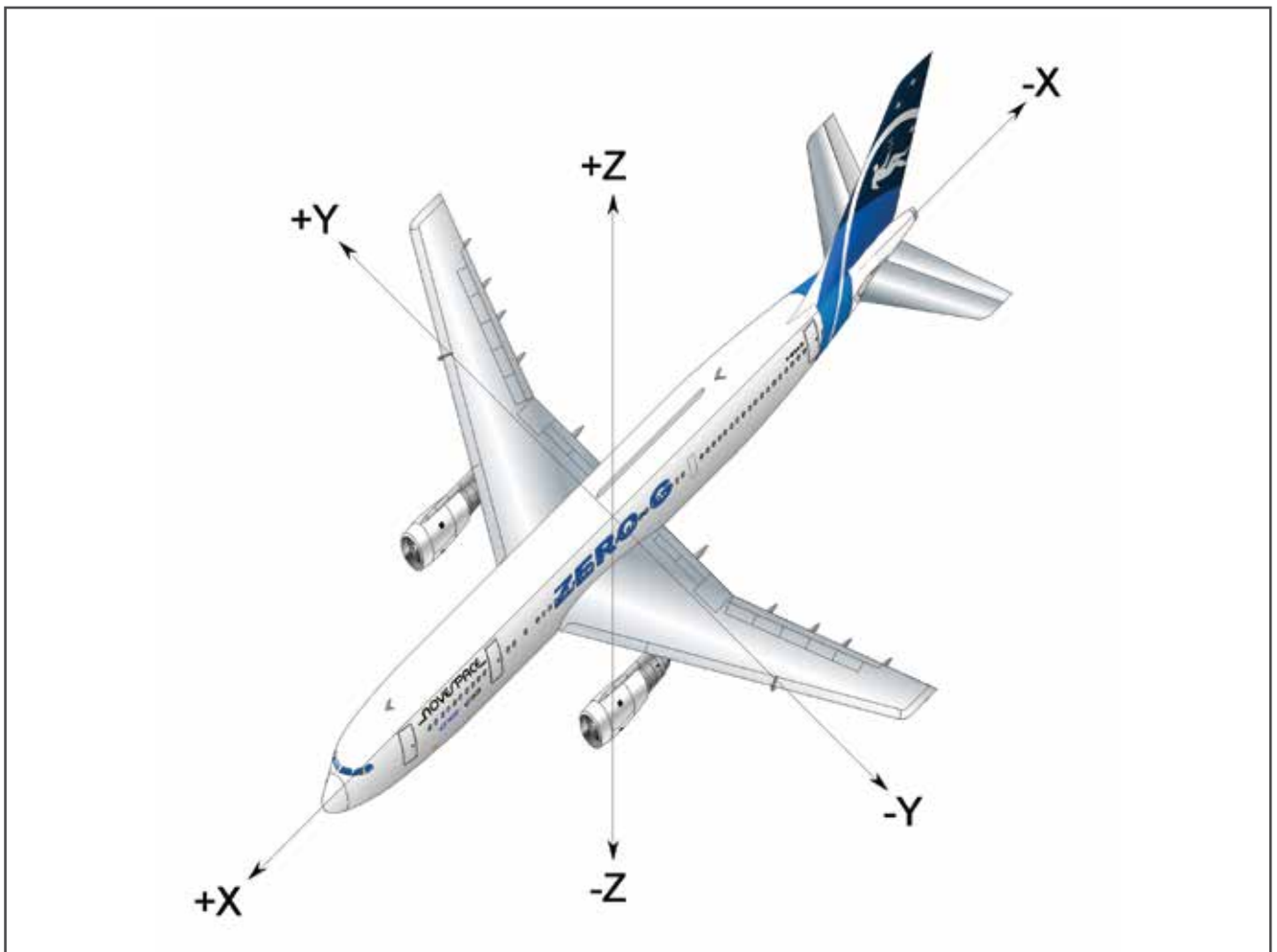
Figure 5-8: Aircraft coordinate reference system
