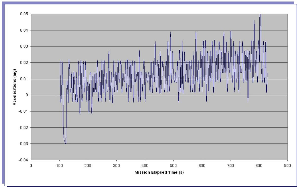
**Figure 5-11: Acceleration (milli g) measured along the flight-path axis during the microgravity phase of the MAXUS 3 mission**
