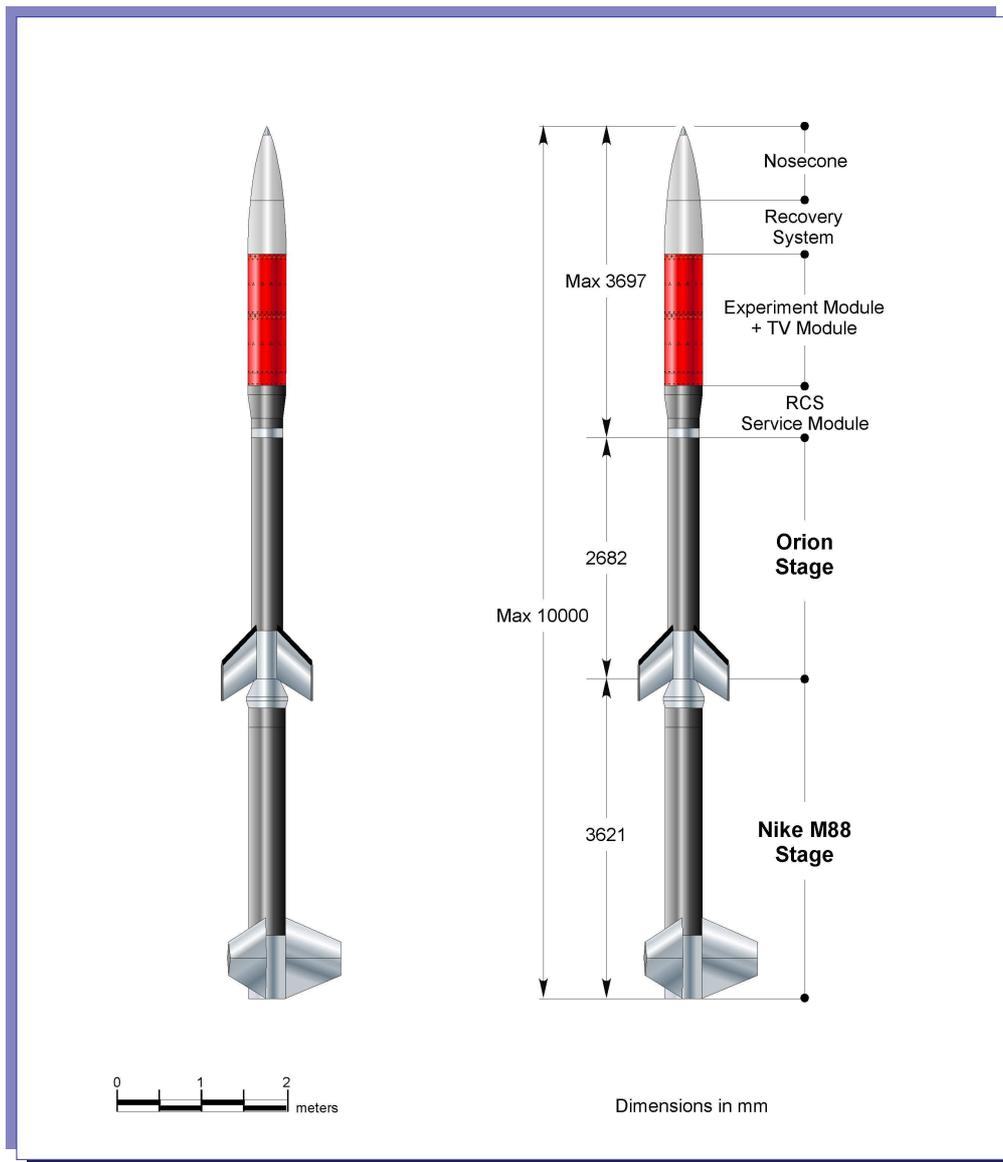
**Figure 5-1: MiniTEXUS sounding rocket**
