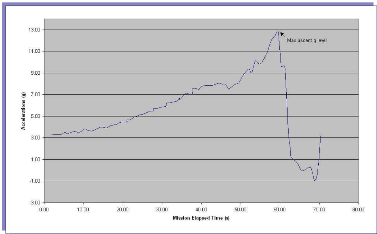
**Figure 5-10: Acceleration (g levels) measured along the flight-path axis during the ascent phase of the MAXUS 5 mission**
