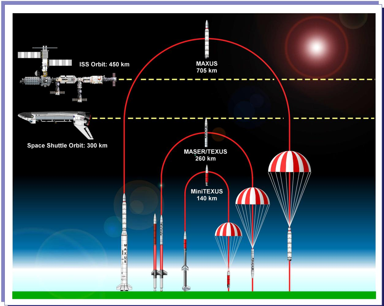
Figure 5-5: ESA sponsored sounding rocket maximum altitudes compared to Shuttle and ISS
