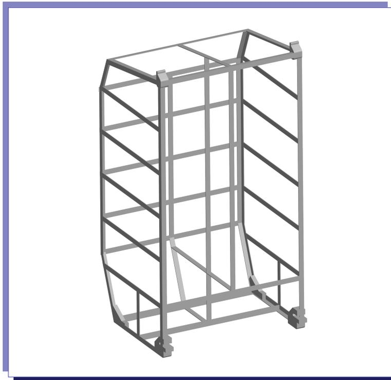
Figure 7-25: International Standard Payload Rack (ISPR): 6-post configuration
