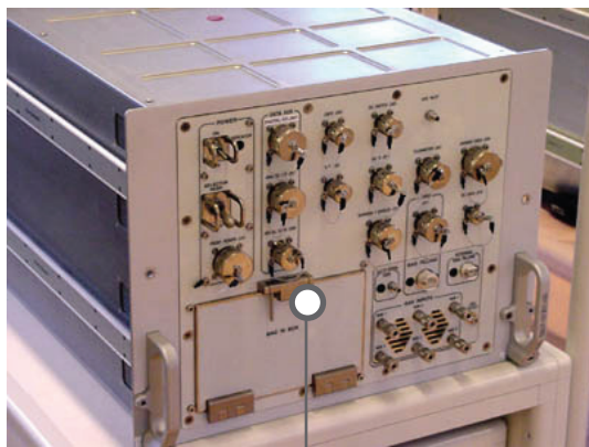
Front panel of the Pulmonary Function System
