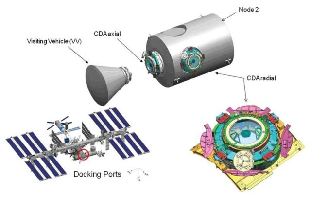
The CDA will be installed on the axial and radial ports of the ISS's Node 2 module to provide a new docking interface for a wide variety of visiting vehicles. Illustration: NASA
