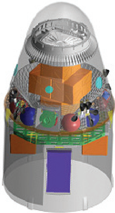
Dragon Spacecraft in Cargo Configuration.
