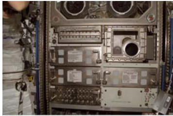
Airlock (right square compartment w. circular hand access) under the MSG, which has a snap-in type of seal, so that area has been the focus of the third leak test.
