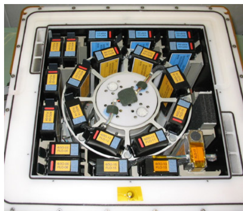
Kubik with centrifuge configuration loaded with experiment containers
