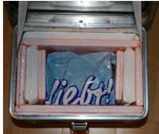
From scientist to Moscow, samples for AT-SPACE And BLOKION are transported inside a passive thermocase with cool packs at 2.8 °C.
