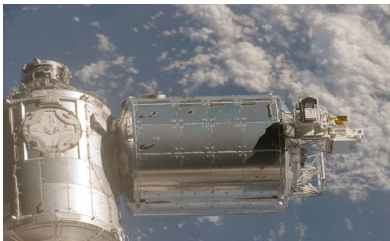
Columbus Module attached: SOLAR (top-right) and EutEF (sticking out to the right) mounted on their structures (courtesy NASA)
