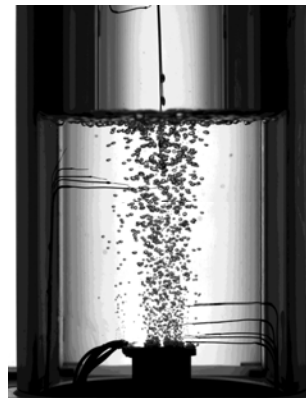
Boiling under normal gravity (lower pict) and under microgravity (top) on MASER-11.
