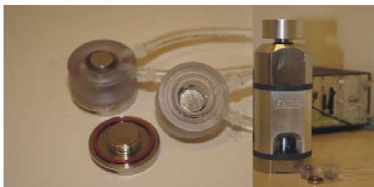
The Zetos bioreactor for culture and mechanical loading (D. Jones)
