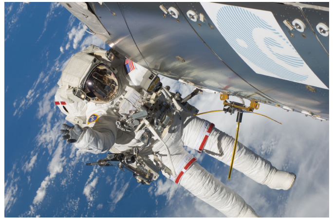
NASA astronaut Randolph Bresnik on 21 November 2009 with the unfurled AIS antenna, attached to Columbus to be used for experimental tracking of VHF signals of ships at sea. Courtesy of NASA.
