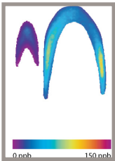
Methane flame under normal- (left) and microgravity (right). Also measured but not shown: temperature, soot volume fraction (shown here), and primary particle diameter. (Courtesy of Reimann and Will)
