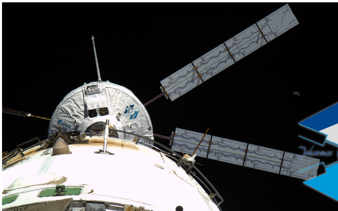
ATV-2 - few meters before docking to the Russian module Zvezda. Part of the navigation alignment system can be seen as two dark square structures above the central circular mating ring of the vehicle. These are visual targets for crew monitoring. Courtesy of NASA.
