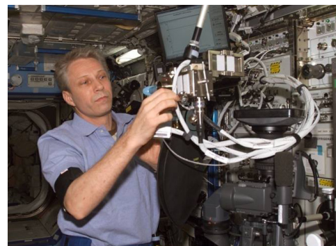
ESA astronaut Thomas Reiter operating the Pulmonary Function System (PFS) in preparation of the CARD experiment. Reiter has experience with an earlier generation of the gas analysers, the RMS-2 which he used onboard the Euromir 95 mission.
