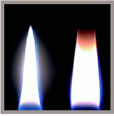
Laminar ethene diffusion flame normal gravity (left) and in microgravity (right) (Courtesy of Reimann and Will)
