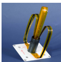
AIS Antenna for ISS before being unfoiled
