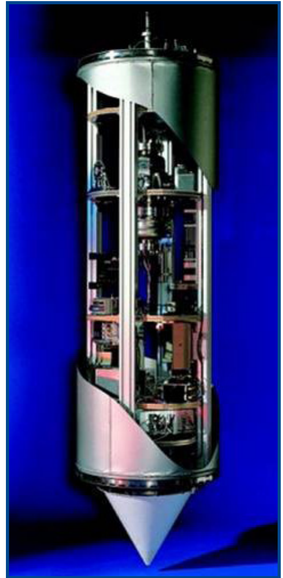
Illustration of the complexity of a fall capsule, here arranged in support of the CPS experiment: Experiment on Combustion Properties of Clouds, Particles and Spray (Courtesy of ZARM)
