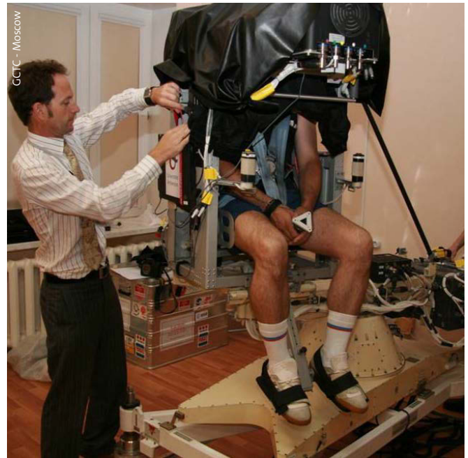
The VVIS rotational chair in Star City near Moscow. Final check before centrifugation of cosmonaut Yuri Malenchenko as part of the Spin experiment
