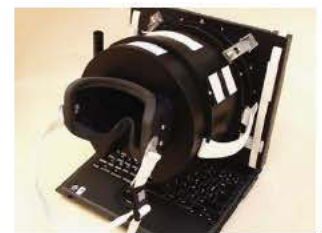
Visual light shield attached to multipurpose laptop through which virtual reality/visual stimuli displayed for specific neuroscience experiments on the ISS. This has included the Passages, Neurospat and older Neurocog experiments
