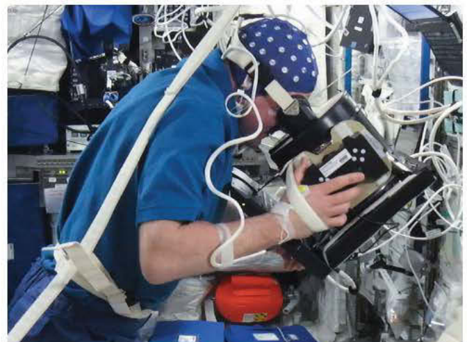
Session of the Neurospat experiment on the ISS in February 2012. ESA astronaut André Kuipers looks through light shield at visual stimuli displayed on attached laptop. At the same time brain activity is monitored through an EEG cap.
