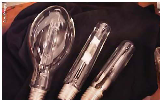
High-Intensity Discharge lamps for the ARGES experiment, one of the experiments for the DELTA Mission in 2004
