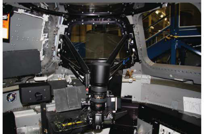
NightPod tracking device installed at a window in the European-built Cupola module
