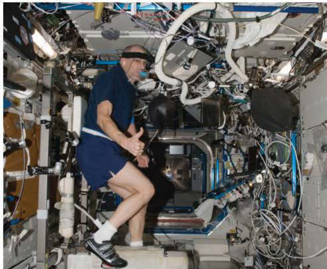
NASA astronaut Don Pettit using the Portable Pulmonary Function System whilst on the CEVIS exercise device during activities for the joint Thermolab/EKE/VO 2 Max experiments
