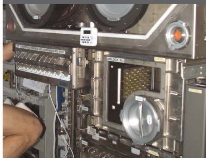
The MSG airlock below the right-hand main astronaut glove port
