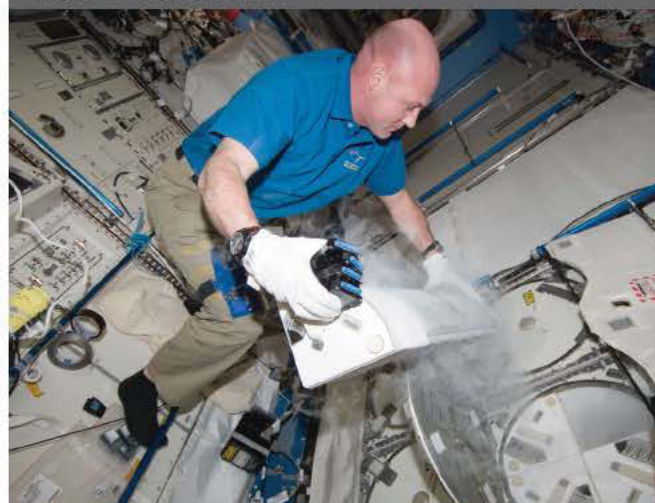
Expedition 30 Flight Engineer and ESA astronaut André Kuipers prepares to insert processed ROALD-2 experiment containers into a European-built MELFI freezer on the ISS in December 2011
