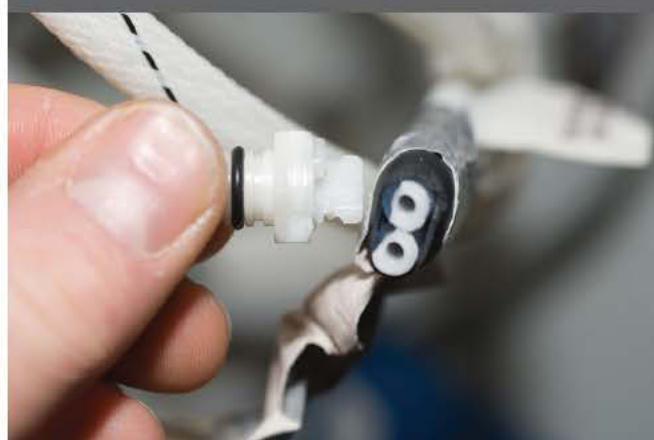
Broken connector during the CARD experiment
