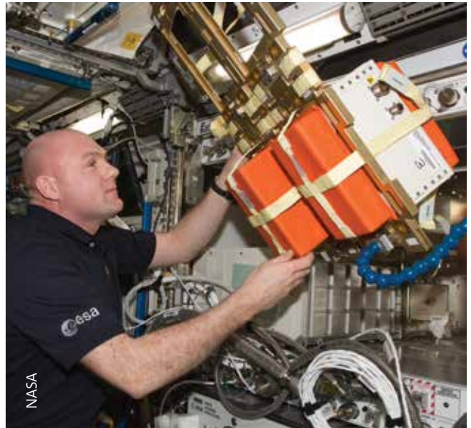
NASA André Kuipers setting up the ALTEA Shield hardware in the Shielding configuration on 8 June 2012
