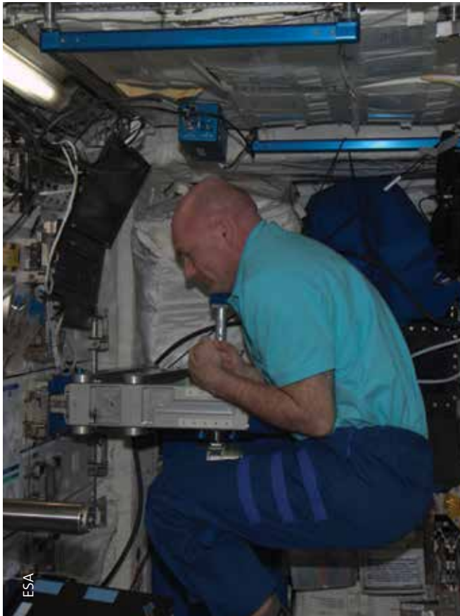
ESA astronaut André Kuipers undertaking Body Mass Measurement for the SOLO experiment on 1 February 2012
