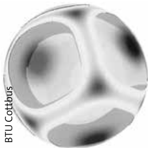
Graphic image generated from a Geoflow numerical model for spherical convective regimes. This octahedral pattern is generated in conditions of no rotation and a medium temperature gradient profile
