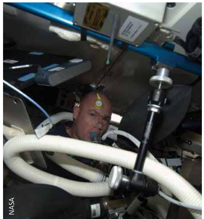
↑ ESA astronaut André Kuipers using the Portable Pulmonary Function System during activities for the joint Thermolab/EKE/ VO 2 Max experiments. Clear view of core body temperature sensor on his forehead
