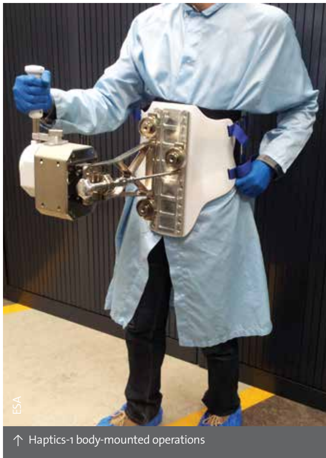
↑ André Schiele, leading ESA's telerobotics lab, demonstrating remote robotic operations wearing an exoskeleton that weighs just 10 kg
