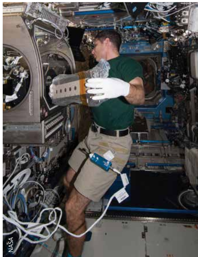
↑ NASA astronaut Michael Hopkins during installation activities in the Microgravity Science Glovebox in November 2013 for the Selectable Optics Diagnostic Instrument - Diffusion Coefficient in Mixtures 2 (SODI-DCMIX 2) experiment
