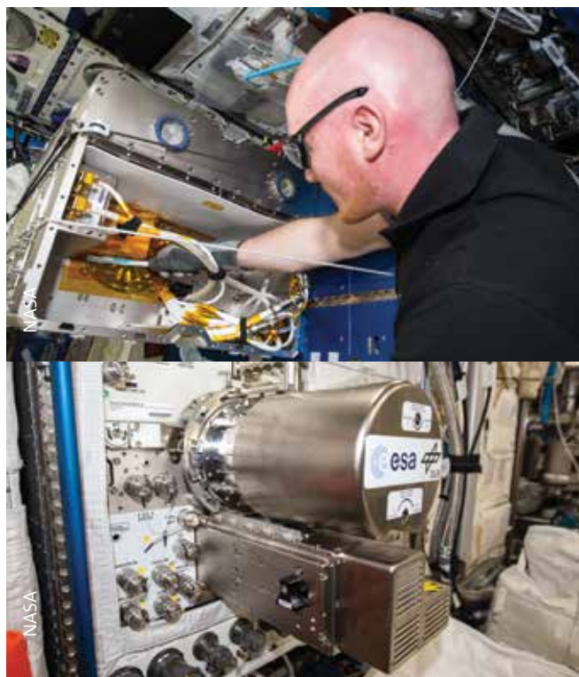
↑ Top: Alexander Gerst undertaking minor troubleshooting too remove a protruding bolt during EML installation procedures in September 2014. Bottom: EML during sample chamber and gas filter installation in October 2014
