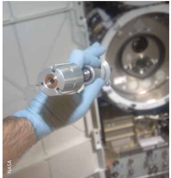
↑ MSL Conical Tool, one of the tools used within the scraping step of the cleaning process of the MSL (in the background)
