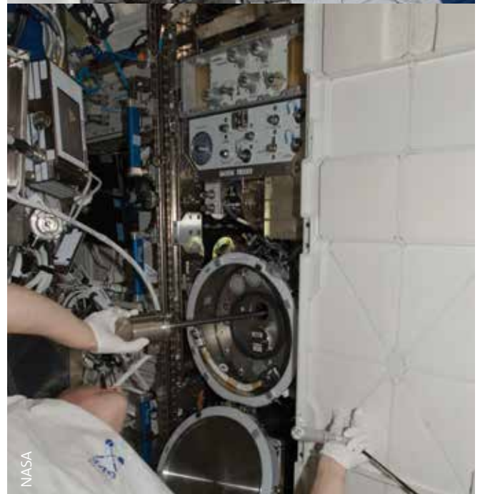
↑ Top: ESA astronaut Frank De Winne installing the Low Gradient Furnace into the Materials Science Laboratory as part of commissioning activities in October 2009. Bottom: De Winne installing a CETSOL sample into the Materials Science Laboratory as part of the first sample exchange on 8 November 2009
