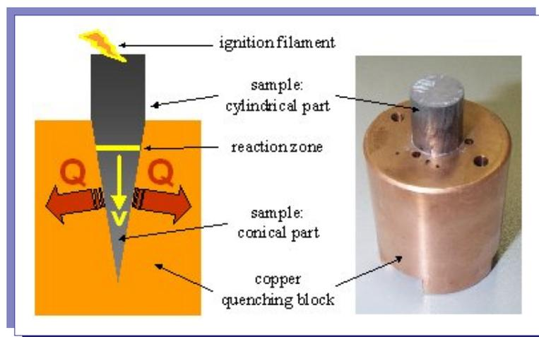
**Figure 2-19: Sample geometry (cylinder coupled with a quenching cone)**
