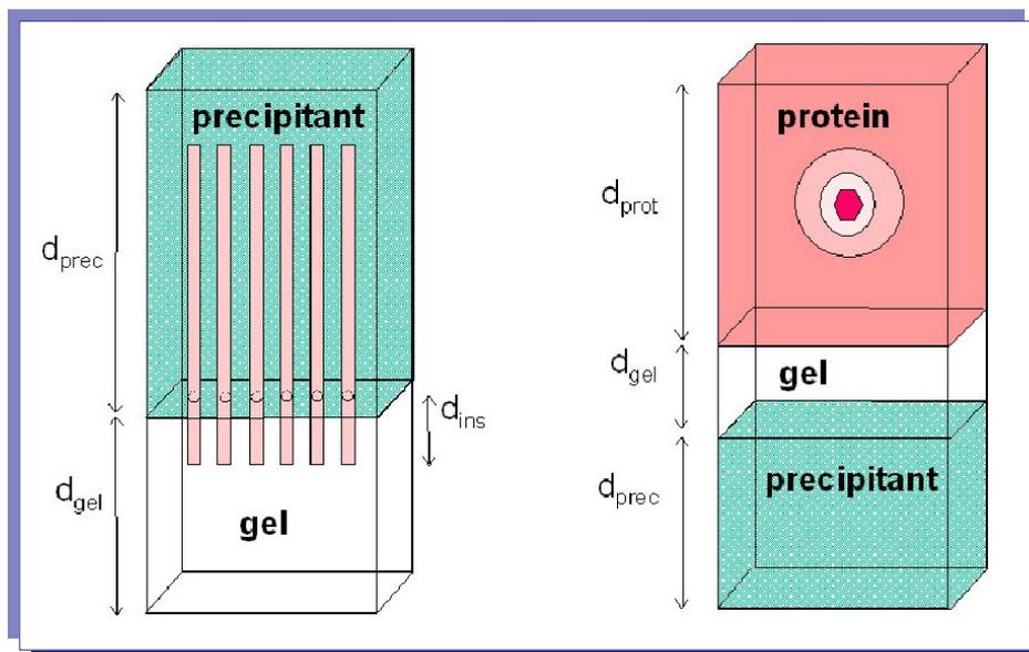
**Figure 2-25: Geometry of the PromISS experiments. Internal volume of the reactors is 52 mm high, 19 mm wide, and 34 mm deep (left: capillary geometry; right: full reactor geometry)**
