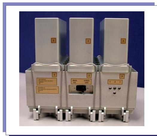
**Figure 2-5: Electronic Control Unit (ECU) with 3 B-containers**
