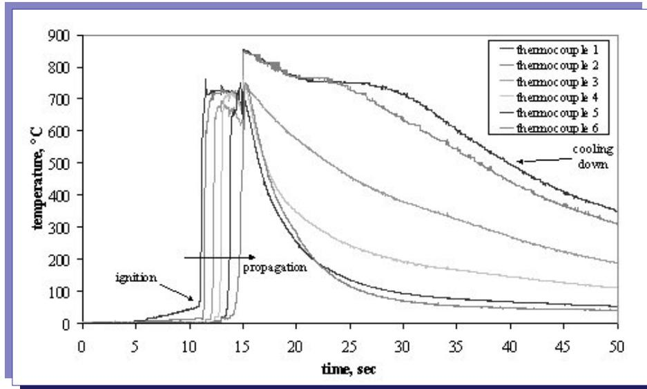
Figure 2-22: Real-time thermocouple data (temperature-time profile) from reactor CSM-ISS-06 (TiAl<sub>3</sub>/TiB<sub>2</sub>)
