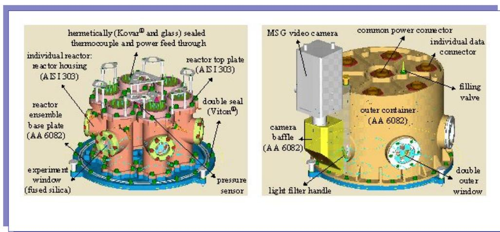
**Figure 2-21: COSMIC reactor ensemble (Left) Inner view; (Right) Outer view**
