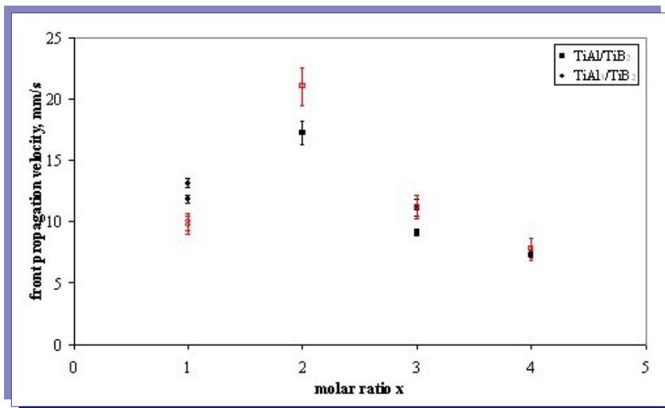
Figure 2-23: Average front propagation velocity in the cylindrical pellet between thermocouple 1 and thermocouple 3 as function of the molar ratio x
