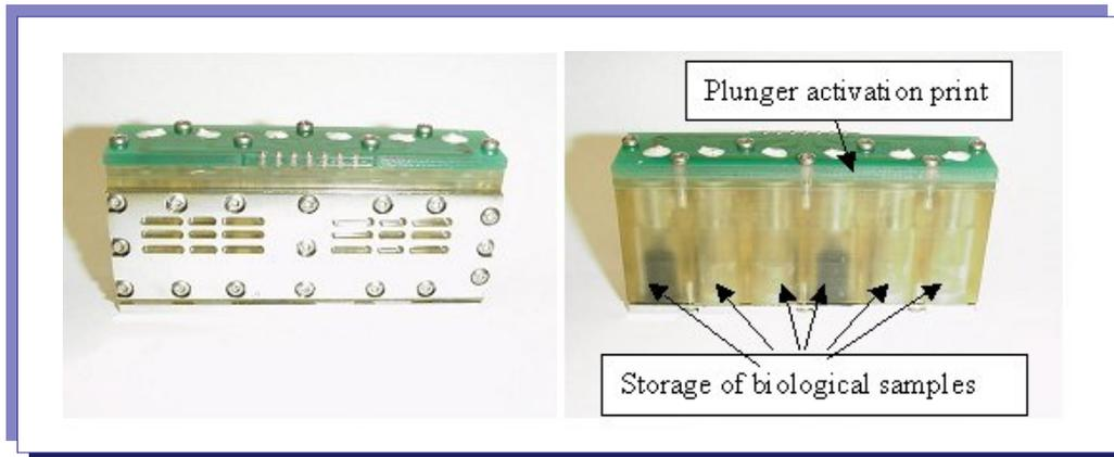
**Figure 2-4: Vitamin D plunger box unit (PBU)**
