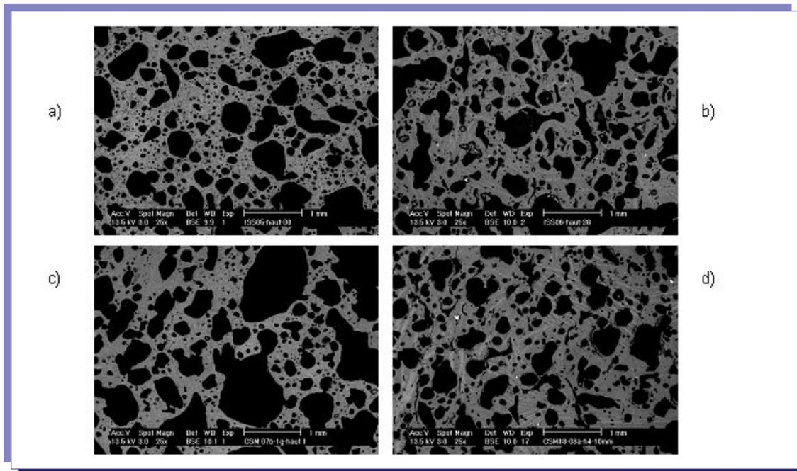
**Figure 2-24: Size and morphology of the porosity at 10 mm from the initial top plane on the axis of the cylindrical part (microgravity samples (a) and (b); ground samples (c) and (d))**
