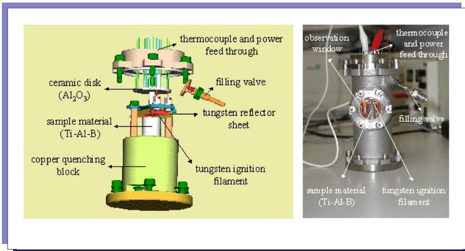
**Figure 2-20: (Left) Inner view of an individual COSMIC reactor showing the main constitutive elements; (Right) External view of a single COSMIC reactor**
