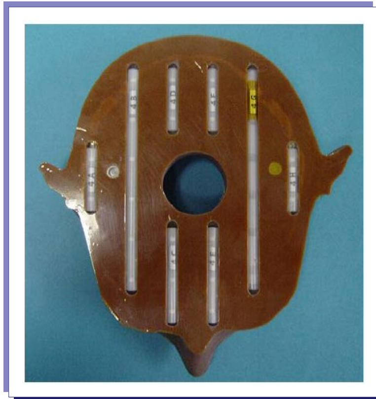
**Figure 2-3: Dosimeter distribution in Phantom Head slice #4**
